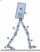
Fig. 5 Sagittal plane representation of BLEEX in the single stance phase.
